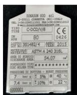
All the essential data of both the manufacturer and the protective device are indelibly marked on the rupture disc or on a metal plate welded to the disc.
