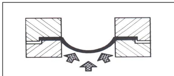
Rupture discs are pressure-tight devices designed to open by means of rupture at a pre-determined pressure value.
