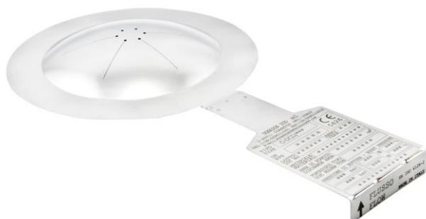
**Conventional (or direct) domed discs (usually to be installed with a disc holder):** The principle adopted to assign a predetermined burst pressure is simply the failure of a metal membrane subjected to a load in its concave part.
