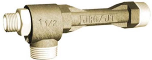
Eductors use the kinetic energy of one liquid to cause another fluid to flow. Eductors consist of a converging nozzle, a body and a diffuser. The converging nozzle converts the pressure energy of the motive liquid to velocity energy. This high velocity liquid flow then entrains the suction liquid. In the body complete mixing of the motive and suction fluids occurs. The mixed fluid is then converted back to an intermediate pressure after passing through the diffuser.
